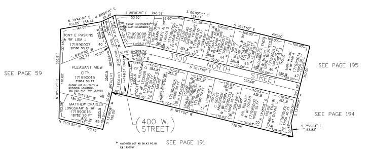
10' UTILITY & DRAINAGE EASEMENTS EACH SIDE OF PROPERTY LINES AS INDICATED BY DASHED LINES EXCEPT AS OTHERWISE SHOWN.
